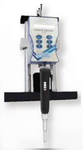
Note: The force gauge is externally calibrated by a third-party laboratory and is verified using standard weights in house.
